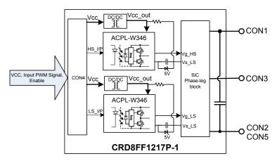
Figure 2. CRD8FF1217P-1 Block diagram with ACPL-W346
