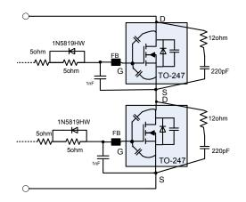
Figure 8. Gate drive and RC snubber configuration
