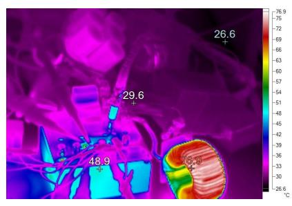
Figure 12. Thermal imaging of the EVL board while under test.
