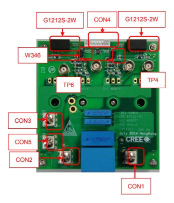
Figure 4. EVL board showing key connectors and components.
