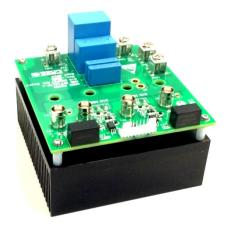
Figure 3. Cree EVL board assembly (see Appendix for assembly instructions).
